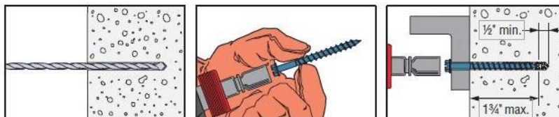
FIGURE 2 – INSTALLATION INSTRUCTIONS FOR TITEN TURBO™ SCREW ANCHORS
