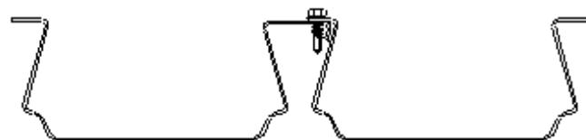
**FIGURE 4.1b - SCREWED SIDE LAP DETAIL FOR TORIS AND TORIS A DECK
