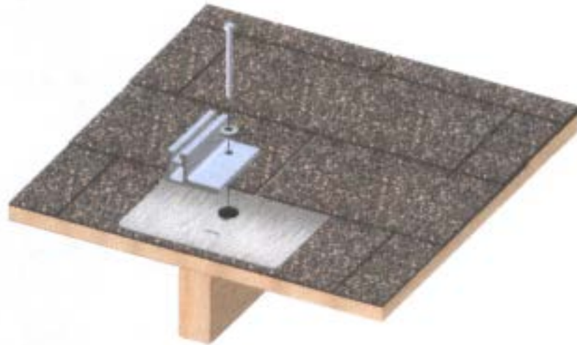
Figure 7: CompSlide Roof Mount Assembly
